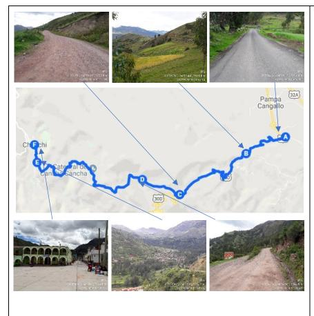
Interventions carried out: Section rehabilitated as nonpaved road under the Rural Project in 2010. In 2014, approximately half of the section was paved under the "Proyecto Peru," an initiative of the Peruvian government, under which they paved several subnational links without changing the road structure or alignment. This was a first step toward a paved road with the recommended width and characteristics when the traffic was enough to justify it.
