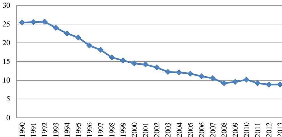
*Note:* In percentage of total domestic generation plus net imports. About one-fourth of the combined losses are incurred in the HV transmission network and the balance in the LV distribution system.
