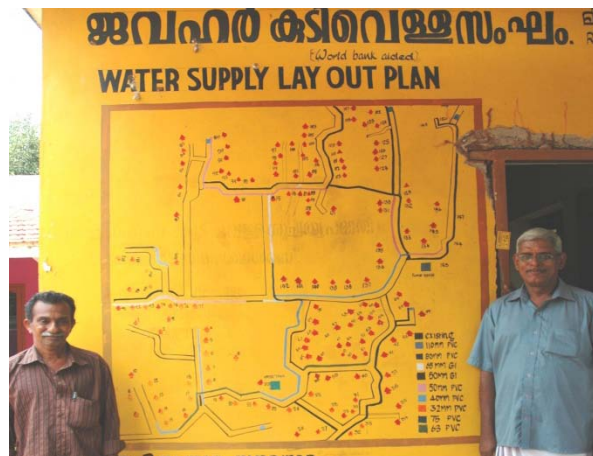
Figure 2. A Typical Small-Scale Kerala Water Scheme Showing Households Connected to the Supply Network
